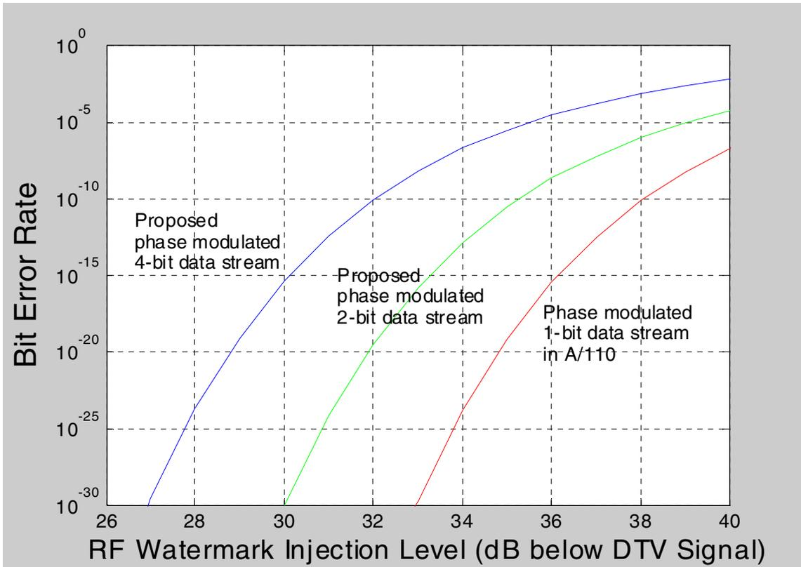
**Figure 2. BER performance vs. watermark injection level for different watermark data transmission systems**
