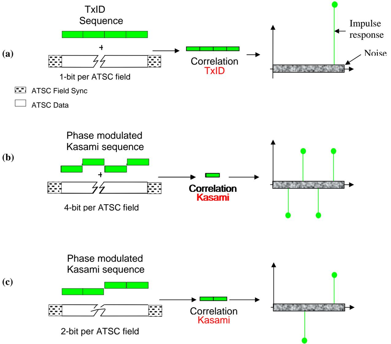
**Figure 1. (a) A/110 RF watermark data transmission system (1 bit per 8-VSB field); (b) Proposed data transmission system with 4 bits per 8-VSB field; (c) Proposed data transmission system with 2 bits per 8-VSB field.**
